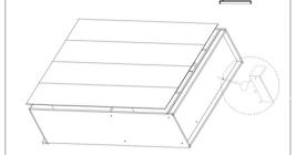
Turn the cabinet carefully to its back and hammer and nails the backs.
