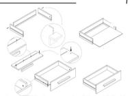
Assemble the drawer on the right and left sides, respectively, to the back of the drawer with cabinet screws. Then pass the backrest. Attach the handle to the front of the drawer with the screw. Then attach minifix shafts to the front of the drawer and mount them to the drawer frame.
