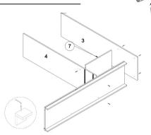
Assemble the side plate number 3, the fixed shelf number 7 and finally the middle pole number 4 on the bottom plate, respectively.
