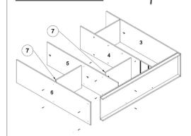
Assemble the fixed shelf number 7, the middle pillar number 5, the fixed shelf number 7 and the side plate number 6, with the logic in step 3.
