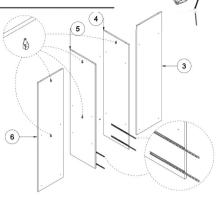
Screw the drawer rails to the doors 4 and 5 using a cordless or screwdriver.
