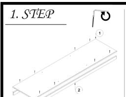
Let's fix the bottom plate number 1 to the bed base number 2 with the help of allen screw and allen.
