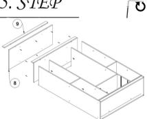
Mount the crown number 9 on the top plate 8, and then fix the top plate on the cabinet.
